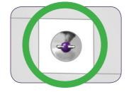
E The sample or reference should also be in contact with **both** port probes.
