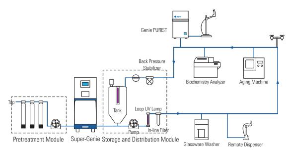
Super-Genie is designed to intergrate centralized water purification system together: from feed water prefiltration devices to distribution loop
