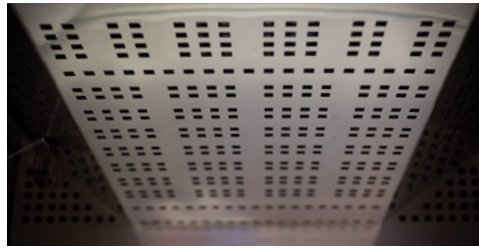
The air baffle forces airflow directly on the product under test, improving product temperature change rates and workspace conditioning.
